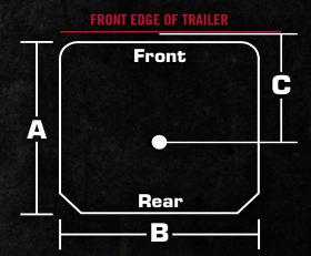
KP Setback = Measurement from the front edge of the trailer to the center of the king pin.
