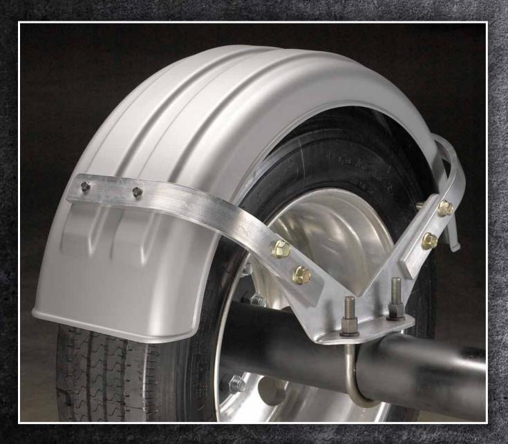
Minimizer Lift Axle brackets are designed specifically for 5" round lift axles. The bracket kit clamps on to the axle allowing the fender to raise and lower with the axle.
