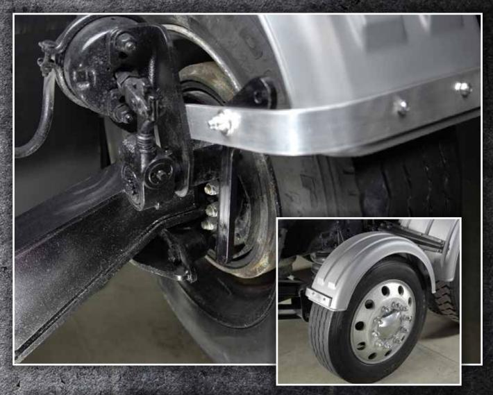
Minimizer Steerable axle brackets bolt on using existing holes on the brake assembly allowing the fender to raise, lower and steer with the wheel.
