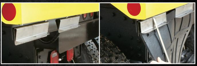
DURABLE - All stainless steel clamp construction, heat tempered to spring steel for ultimate durability.
