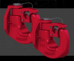
Max Gross Trailer Weight: 30,000 lbs. (13,607 kg) Maximum Tongue Weight: 4,500 lbs. (2,041 kg) Ultimate Latch Capacity: 5,000 lbs. (2,267 kg) Maximum Eye X-Section: 1 13/16 in. (46 mm) Minimum Eye Opening: 2 in. (51 mm) Unit Weight: 14 lbs. (6.4 kg) - Uses 1/2" mounting holes
