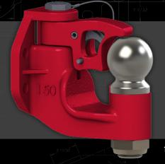
MGTW with Drawbar Eye: 20,000 lbs. (9,072 kg) MGTW with 155 or 156 Ball: 10,000 lbs. (4,535 kg) Maximum Tongue Weight: 2,500 lbs. (1,134 kg) Ultimate Latch Capacity: 5,000 lbs. (2,267 kg) Maximum Eye X-Section: 1 13/16 in. (46 mm) Minimum Eye Opening: 2 3/8 in. (60 mm) Unit Weight: 15 lbs. (6.8 kg)
