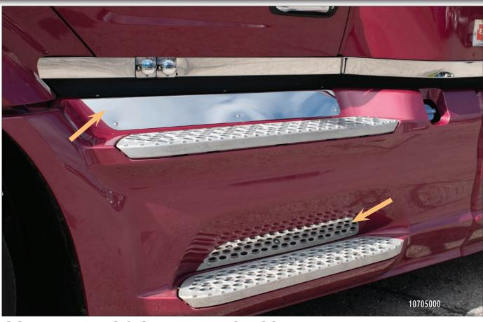
**SCUFF PANELS & STEP DPF BOX COVER**For models with fairings. Add a layer of protection with these high-quality 304 stainless steel panels. Attach using supplied hardware and 3M two-sided tape. Sold in sets (upper & lower for both passenger and driver sides).
