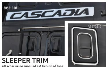
Attaches using supplied 3M two-sided tape.
