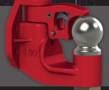
MGTW with Drawbar Eye: 20,000 lbs. (9,072 kg) MGTW with 155 or 156 Ball: 10,000 lbs. (4,535 kg) Maximum Tongue Weight: 2,500 lbs. (1,134 kg) Ultimate Latch Capacity: 5,000 lbs. (2,267 kg) Maximum Eye X-Section: 1 13/16 in. (46 mm) Minimum Eye Opening: 2 3/8 in. (60 mm) Unit Weight: 15 lbs. (6.8 kg)
