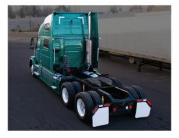
Low-profile, single layer design provides resistance to peeling or impact from debris during use.
