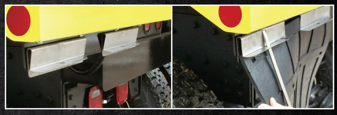
DURABLE - All stainless steel clamp construction, heat tempered to spring steel for ultimate durability.
